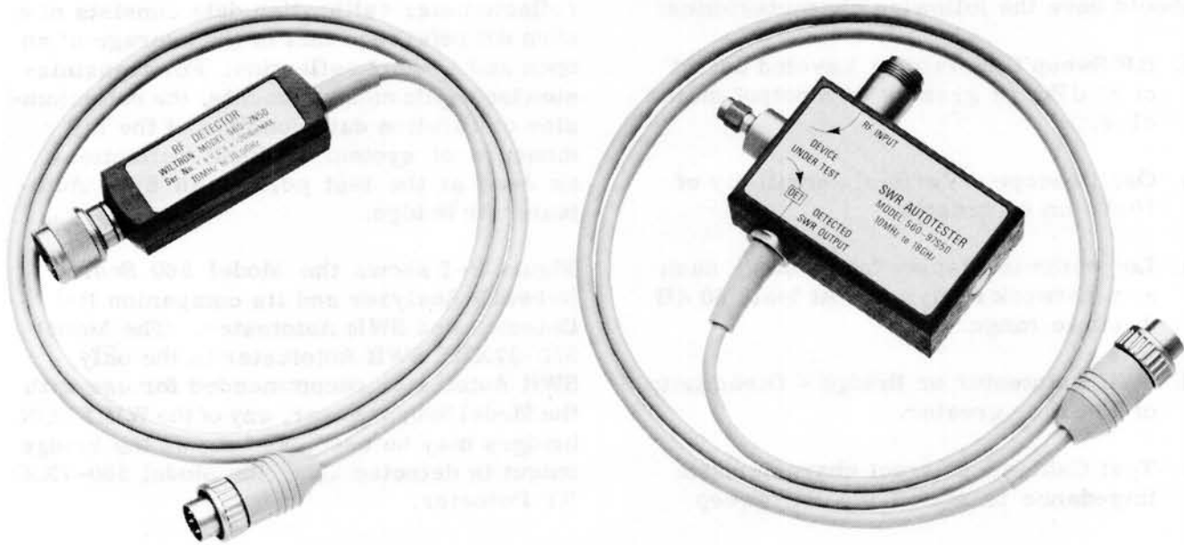
Figure 2-1. Model 560 Scalar Network Analyzer With Companion RF Detector and SWR Autotester
